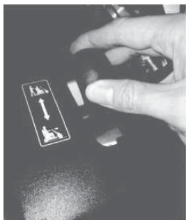
Disengage and in freewheel mode.
